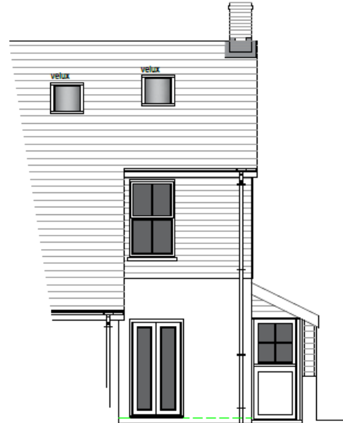
part existing rear elevation
